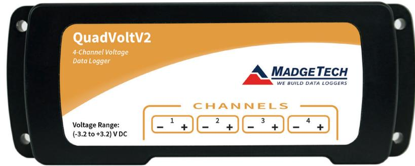
The QuadVolt V2 is an 4-channel, battery powered, DC voltage data logger with a reading rate of up to 4 Hz. It can measure and record 349,184 readings per channel. To maximize memory capacity, users can enable or disable channels. For easy identification, each channel can be named with up to a ten digit title.
