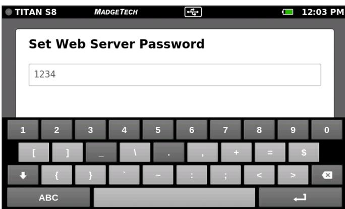
Certain keys are disabled on the numeric virtual keyboard. The User ID and Password may only consist of characters that are considered "URL safe". Select the Up/Down (Shift) arrow to access additional special characters. Select **Enter** key when finished entering the User ID.
