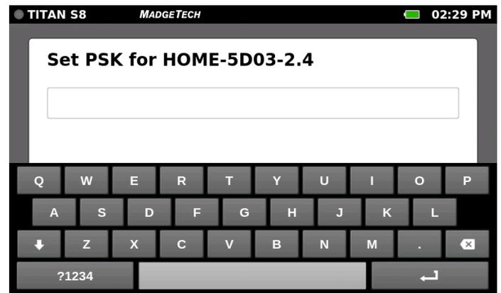
Enter the Wi-Fi SSID password which can be any character on the virtual keyboard displayed on the Titan S8 screen. Space and double quote characters are not permitted for the PSK.
