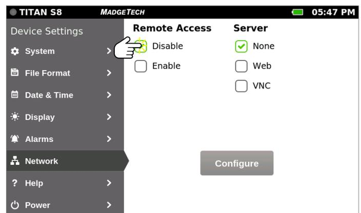
Select Remote Access **Disable** checkbox to disconnect the Ethernet connection to proceed with setting up the Web Server Configuration on the next page.
