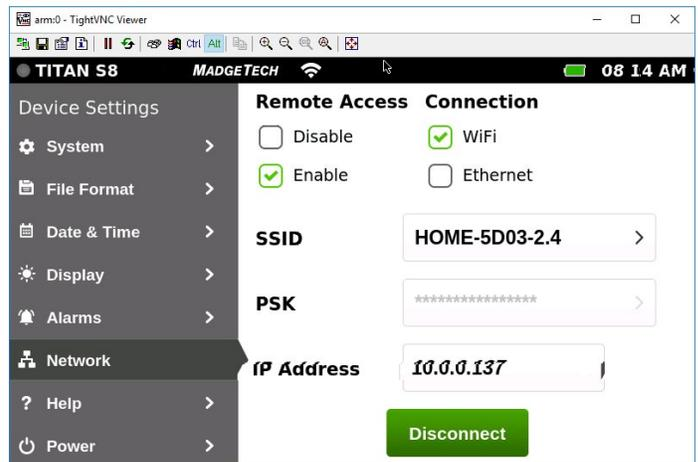
After the network connection is made an arrow pointer will appear on the TightVNC screen and on the Titan S8 screen. The VNC Viewer does not need to be running for the arrow pointer to appear on the Titan S8 screen. If the local Titan S8 arrow pointer moves on its own, the device is being remotely controlled.
