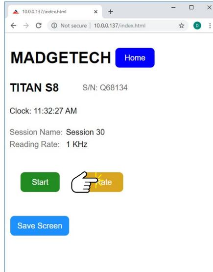
**Home > Start Logging >** From the **Start Logging** page, the remote user can click the **Rate** button to change the Reading Rate on the device.
