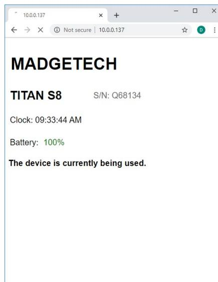
When this message is displayed, the local user is currently using the device or not enough time as passed since the local user has used the device. The local user always has priority using the device over the remote user.
