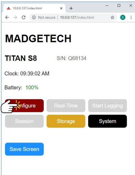
**Home >** Once the remote user has access to the Titan S8 device, the remote user can use the six main Home screen buttons. Click the **Configure** button on the Home Screen to reach the Channel Configuration screen on the Titan S8 device.
