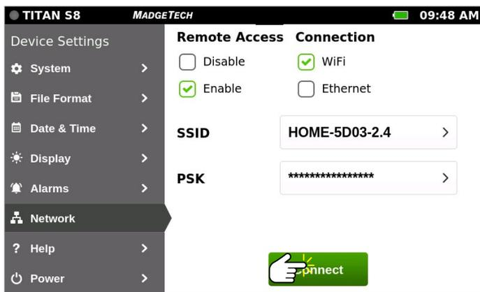
Select the checkbox for either the Wi-Fi or Ethernet connection that was previously set up. Select **Connect** to enable either Wi-Fi or Ethernet connection. See **page 2** for steps to configure the Wi-Fi connection and **page 5** for steps to configure the Ethernet connection.
