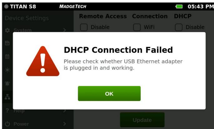
Error message will be displayed if the DHCP connection fails. Similar message will be displayed if the Ethernet static connection fails.
