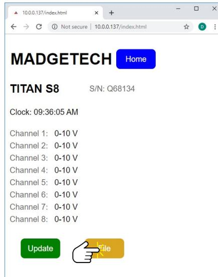
**Home > Configure >** The remote user cannot access or see everything on the web browser that the local user can see or do directly on the device. For example, the remote user cannot directly configure a channel. However, the remote user can press the **File** button to reach previously saved channel configurations on the device.
