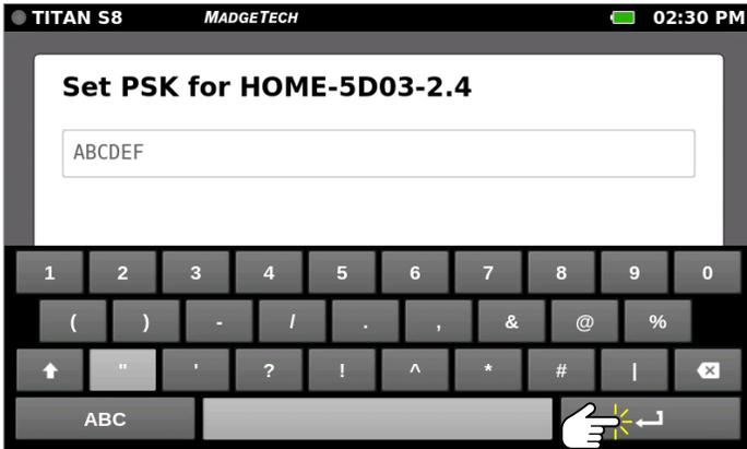
Select the ?1234 button to type in special characters and numbers. Select the Up/Down (Shift) arrow to access additional special characters. Press the **Enter** key to exit to the next screen.
