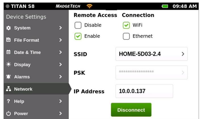
If the network connection is successful, the network icon for either Wi-Fi or Ethernet is displayed on the Top Bar of the screen.
