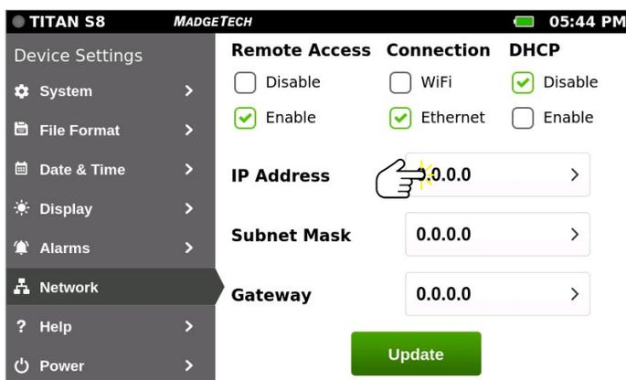
To manually enter the IP Address, Subnet Mask, and Gateway, select the **Disable** checkbox. To enter the IP Address, press the **IP Address** text box.
