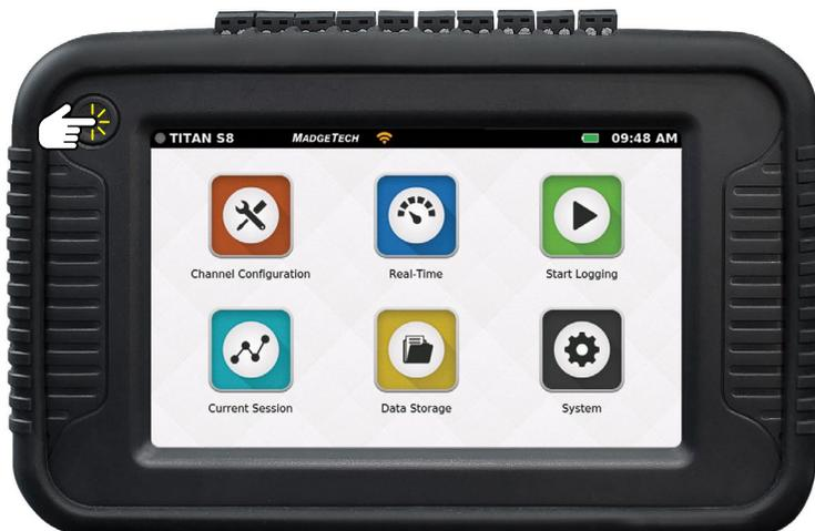
**NOTE:** Press the Home button on the Titan S8 device to return to the Home Screen in order to remotely view or control the device.
