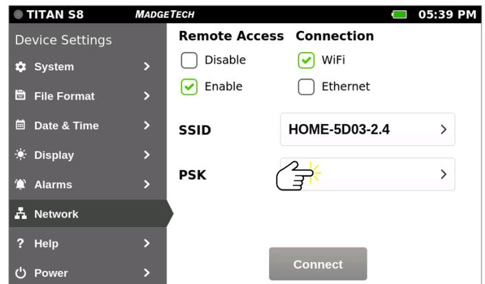
Press the PSK text box to set the Wi-Fi SSID password.
