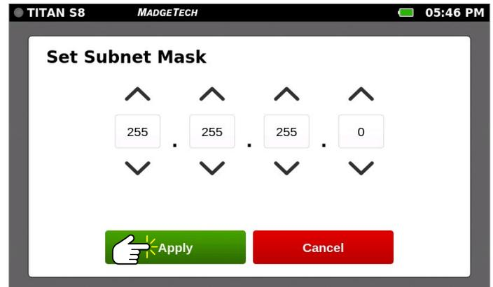
Set the Subnet Mask by pressing the up and down arrows to select the numbers. Hold down the arrows to quickly scroll through the numbers. Select **Apply** to accept the Subnet Mask.
