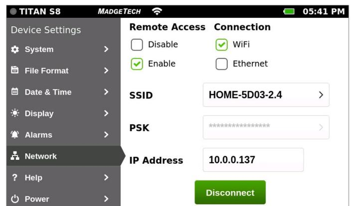
Until a server is selected, you will not be able to view or control the Titan S8 remotely. To connect the Titan S8 to a server using a Wi-Fi connection, see the Open Web Server Configuration on [page 8](#).
