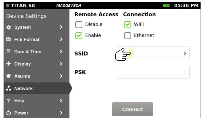
1. Set the Remote Access by selecting the **Enable** checkbox.
