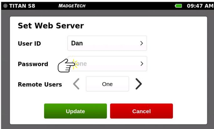
Press in the **Password** text box to bring up the virtual keyboard.
