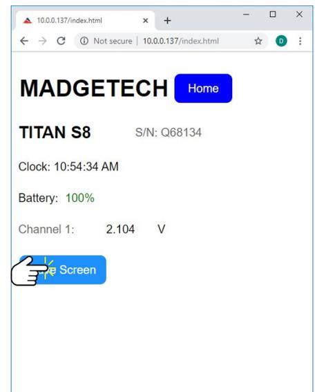
**Home > Real-Time >** Zero values will be displayed for a few seconds before the real data values are displayed. To see what is being displayed on the Titan-S8 screen, click on the **Save Screen** button to download a screen shot to your computer.
