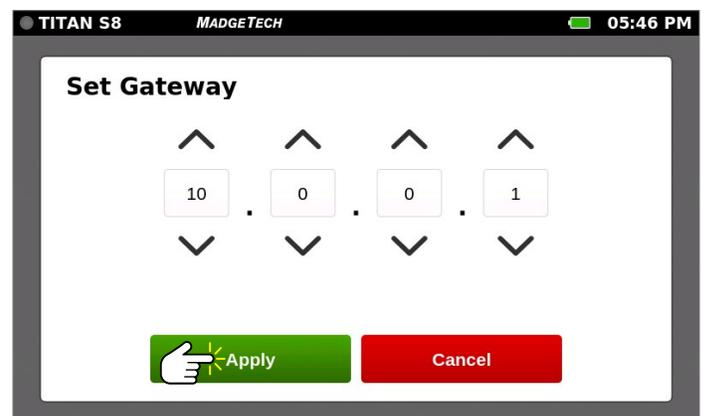
Set the Gateway by pressing the up and down arrows to select the numbers. Hold down the arrows to quickly scroll through the numbers. Select **Apply** to accept the Gateway.
