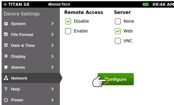
Select **System** from the Home screen and then **Network** if not already on this screen. Select **Web Server** and **Configure** to configure the server. Make sure Remote Access is set to **Disable**.
