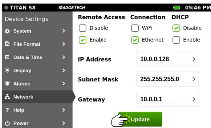
Select **Update** to make the static Ethernet connection. If Ethernet connection is successful, the network icon will be displayed on the Top Bar. Continue to next section to configure the web server to view or control the Titan S8 remotely.
