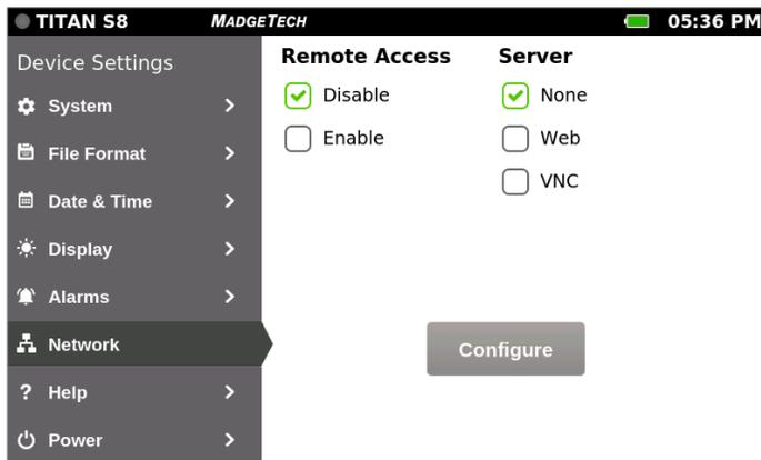
The supported servers can only be configured when **Remote Access** is set to **Disable**. Setting the Web Server is covered on [page 8](#) and the VNC Server on [page 16](#). For now, select **None** as the server type to get started.
