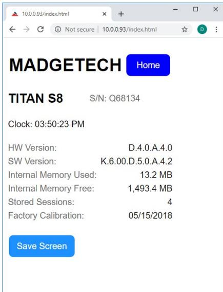
**Home > System >** From the **Home** page, click the **System** button to view limited system information. The remote user does not have access to all the information and buttons on the Titan S8 System screen.
