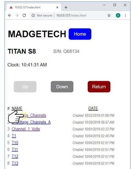
**Home > Configure > File >** Scroll up/down to select one of the channel configurations previously saved on the device. Click a saved channel configuration to change to a new channel configuration.
