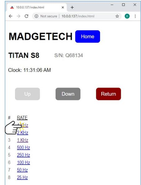
**Home > Start Logging > Select New Reading Rate >** Change to new reading rate.
