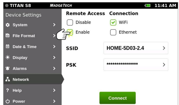
Once the Titan S8 device has been restarted, go to **Settings > Network**, select the Remote Access **Enable** checkbox and select **Connect** to turn back on wireless connection in order to connect to the VNC Viewer.
