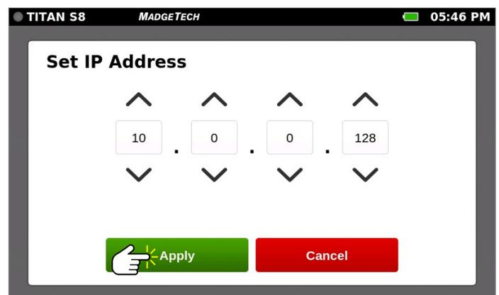
Set the IP address by pressing the up and down arrows to select the numbers. Hold down the arrows to quickly scroll through the numbers. Select **Apply** to accept the IP Address.
