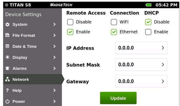
1. Set the Remote Access by selecting **Enable** checkbox.
