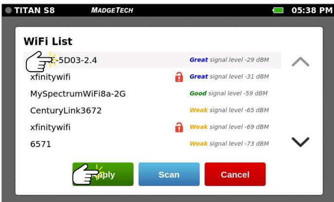
After scanning, the available SSID's are displayed. The red open lock means the Wi-Fi SSID is not secured with a password. The list is sorted by signal strength with the strongest signal at the top of the list. Any hidden SSID will not show up in this list.
