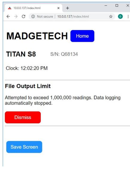
There are other Titan S8 warnings that the remote user can dismiss. There will be a slight delay before the remote user is allowed to dismiss the warning, so the local user has a chance to see the same warning.
