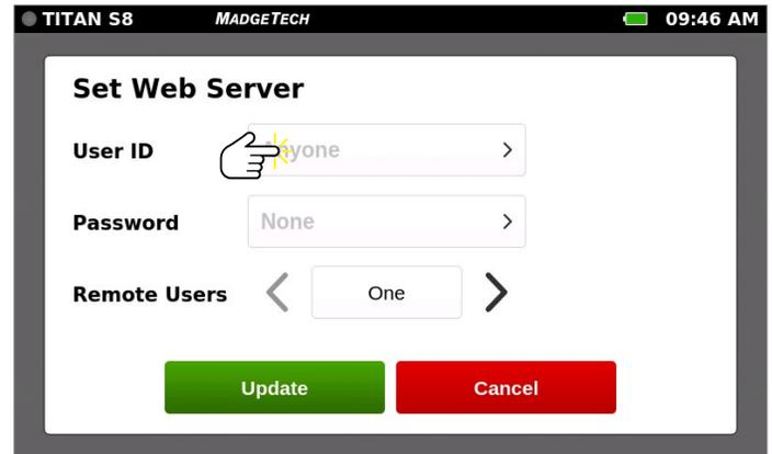
The default user ID on the web server is Anyone and the password is None. It is highly recommended to change these settings to restrict remote access from unauthorized users. Select the **User ID** text field to change the User ID.
