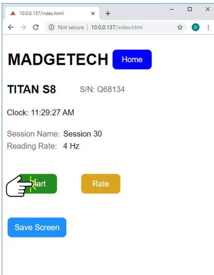
**Home > Start Logging > Select New Reading Rate > Start >** The reading rate was changed to 1 KHz from 4 Hz. Click the **Start** button to start data logging and return to the Home Screen.
