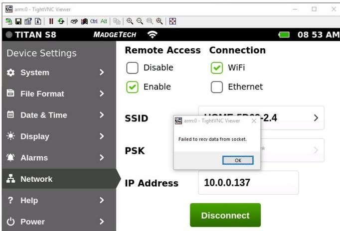
The remote user cannot change the VNC Server password because Remote Access has to be disabled. Disabling Remote Access breaks the VNC Server to VNC Viewer connection.
