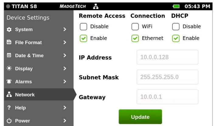
The IP Address, Subnet Mask, and Gateway will display if the connection is successful. These values are not changeable.
