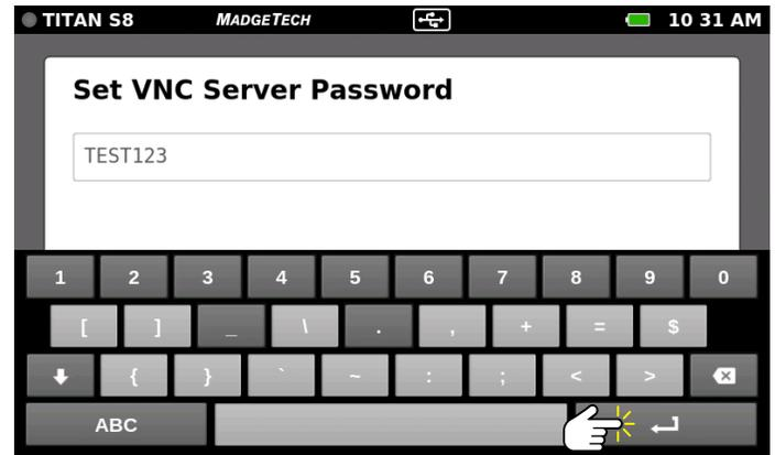
Press in the text box to bring up the virtual keyboard. Some keys are disabled as those characters are not permitted in the Password. Select the Up/Down (Shift) arrow to access additional special characters. The VNC Server Password must be over five characters. Select **Enter** key when finished entering the Password.
