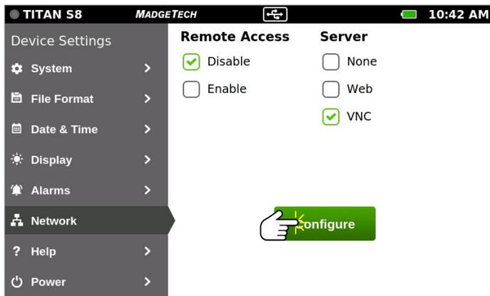
Select **System** from the Home screen and then **Network** if not already on this screen. Make sure Remote Access is set to **Disable**. Select **VNC Server** and **Configure** to configure the server.
