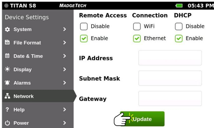
Set the DHCP by selecting the **Enable** checkbox. Select **Update** to attempt to fill in the IP Address, Subnet Mask, and Gateway automatically.
