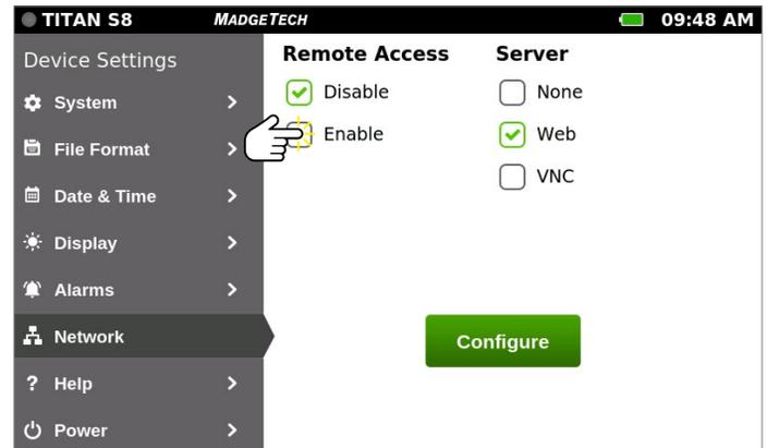
Once the Web Server has been configured, select the Remote Access **Enable** checkbox to test the Web Server network connection.
