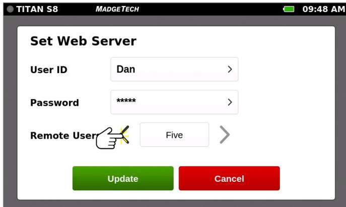
Use the left and right arrows to select the number of remote users that can control the device at the same time. Select **Update** to finish configuring the Web Server.
