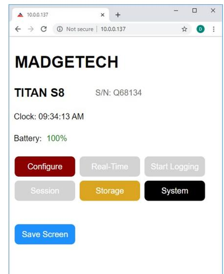
More than one remote user can simultaneously be logged into the same Titan S8 device. The device can be configured to support up to five remote users. See **page 8** for instructions.
