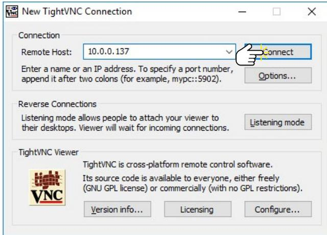
Download and install VNC Viewer (TightVNC is being used in these for this demonstration). Using the configured IP address of the Titan S8 (see [page 4](#) for Wi-Fi and [page 6](#) for Ethernet), enter it into the Remote Host text box. The IP address must match the IP address of the Titan S8 device. Click **Connect**.
