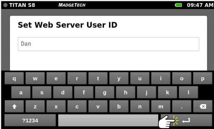
Additional keys are disabled on the numeric virtual keyboard. The User ID and Password may only consist of characters that are considered "URL safe". Select **Enter** key when finished entering the User ID.
